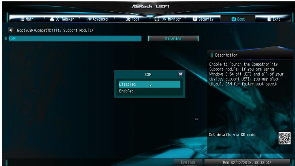
3. After adjusting above option, press “F10” to save the configuration.
