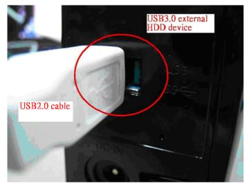
Please connect USB3.0 cable on USB3.0 external HDD device to run at SuperSpeed mode.
