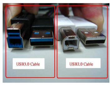
If you connect USB2.0 cable on USB3.0 external HDD device like below, it will not run at SuperSpeed mode.
